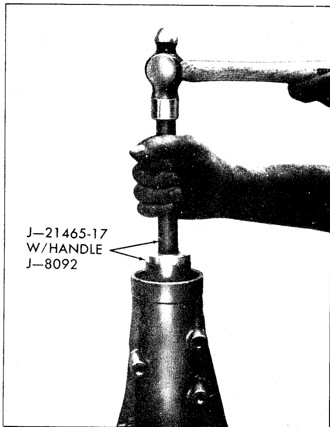
Fig. 7B-14K--Removing Rear Extension Bushing
